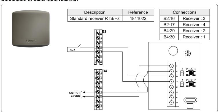
d≥: Step by step command allows to control the shutter from a SIMU remote control (installation of standard receiver RTS/HZ below).
