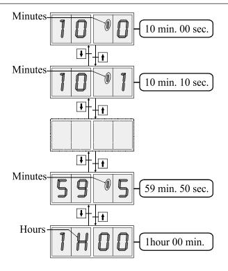
Between 1 min and 10 min press the button 1 or 1 or to increase or decrease the timer by 5s.
