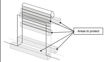
Risk of crushing between the ground and the lower edge of the door during closing.
